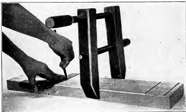
Fig. 194—Legs Clamped for Lining
